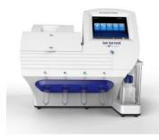
My instrument is based on a similar principle, but sequencing occurs in real time. First, briefly on how semiconductor sequencing occurs. The entire DNA strand is divided into fragments of 300-400 nucleotides in length, called reads. Then the reads attach to small spheres and are copied many times - as a result, a whole bunch of identical DNA fragments hangs on each sphere. Copying is necessary to enhance the signal from each particular read. A set of different spheres is called a DNA library.
